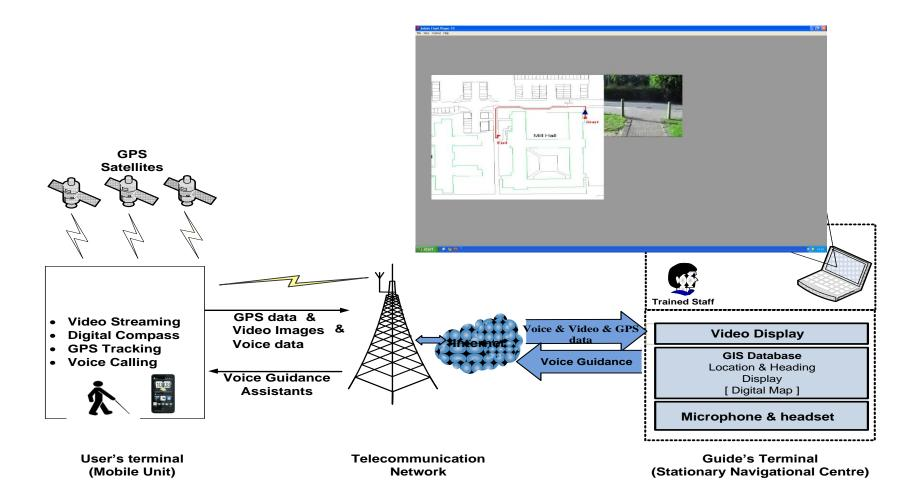
*Figure 3. 1 Brunel remote guidance system prototype*
