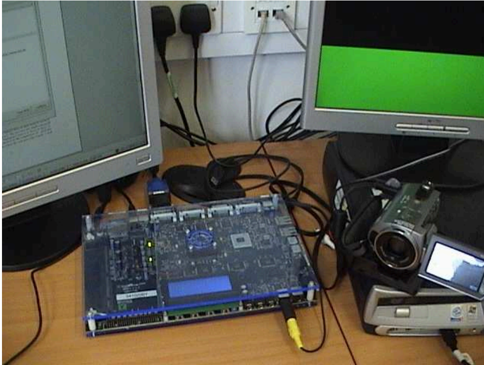
Fig. 10. The system setup includes a Celoxica RC340 board, a digital camera and two monitors. The modified LGMD model lights up the LEDs (flash lights) on the FPGA board based on the values of both LGMD and D cells. These values are also shown on the LCD of the FPGA board.
