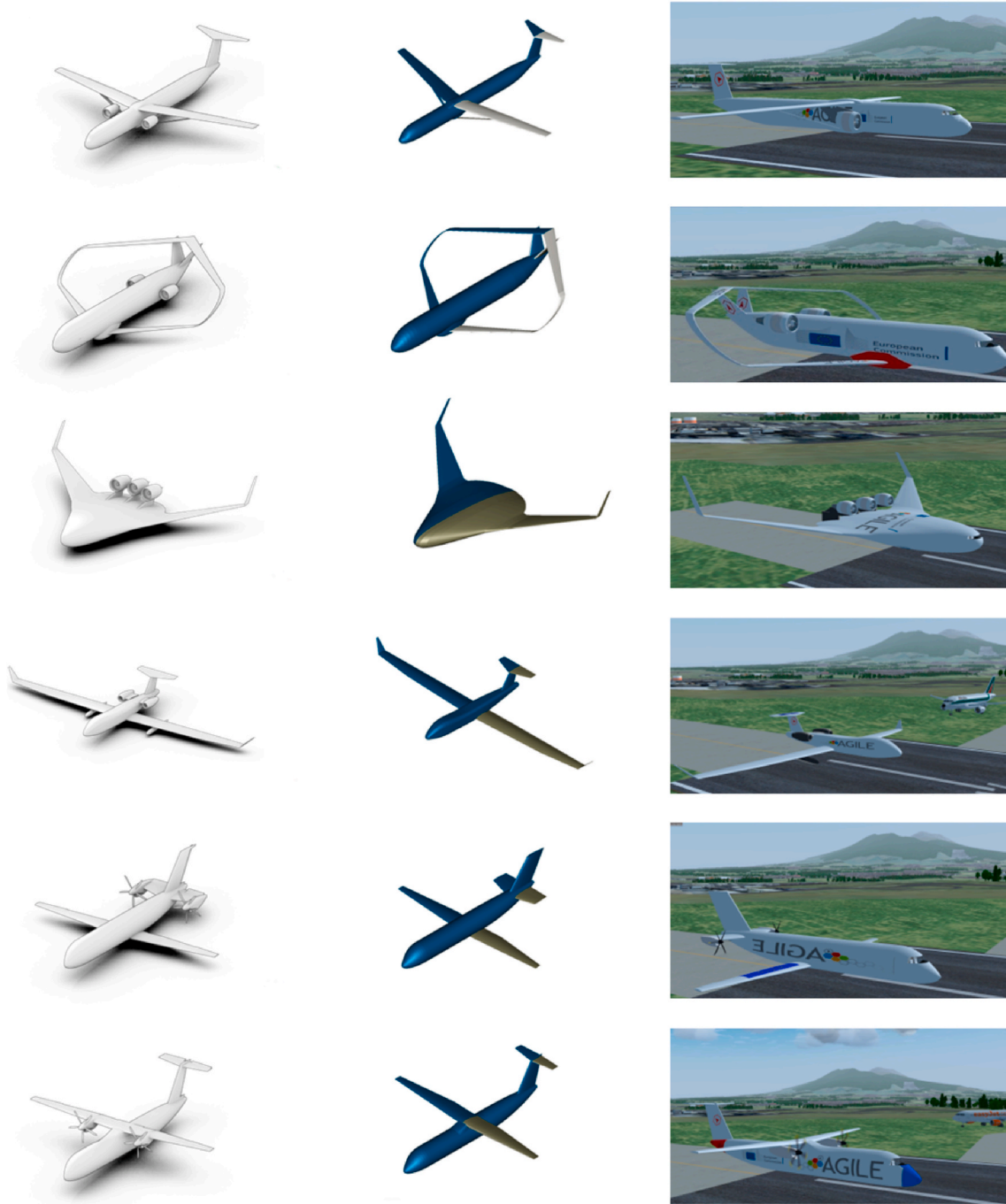
Fig. 25. AGILE Novel configurations (left) available in the database and corresponding CPACS models (middle) and FlightGear models (right).
