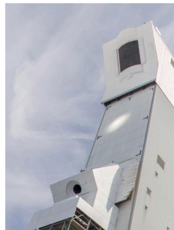
Fig. 1. Illustration of the camera-target method by Stone (1986) (left), Example of a Lambertian target with a solar focus during a calibration procedure at the Solar Tower Jülich, Germany (right). (Photo: DLR, CC-BY 3.0)
