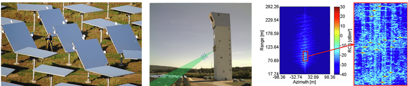
Fig. 12. Exemplary measuring scene of five heliostats equipped with three corner reflectors at the Solar Tower Jülich (STJ) (left), Position of radar on the research platform of the STJ (middle), Processed SAR image of heliostat field with five heliostats in the centre, each is equipped with three corner reflectors (right) (Sauerborn et al., 2012).
