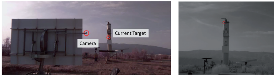
Fig. 21. Heliostat with mounted camera viewing an artificial light target on a tower during calibration (left), View of an artificial light target as seen by a camera mounted to a heliostat (right). The targets as well as camera are highlighted with red circles. Reprinted from Burisch et al. (2018a), with the permission of AIP Publishing.
