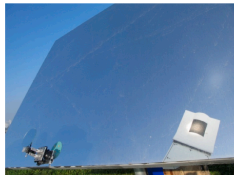
Fig. 8. Illustration of method described by Flesch et al. (2012), Gross (2016) and Belhomme et al. (2011) (left), A small mirror attached to a heliostat at the Solar Tower Jülich as a test setup (right) (Flesch et al., 2012).
