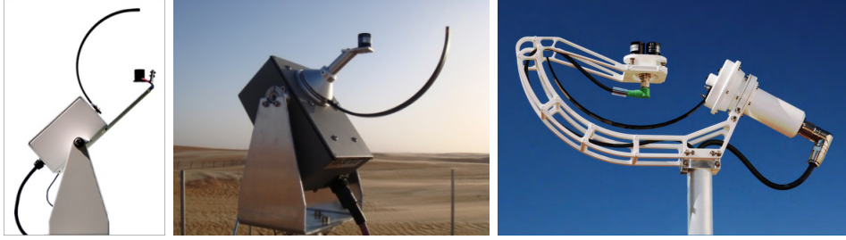
Figure 2.6: Rotating Shadowband Irradiometers. Left: RSR2, center: RSP4G, right: Twin-RSI. [Wilbert et al., 2014]
