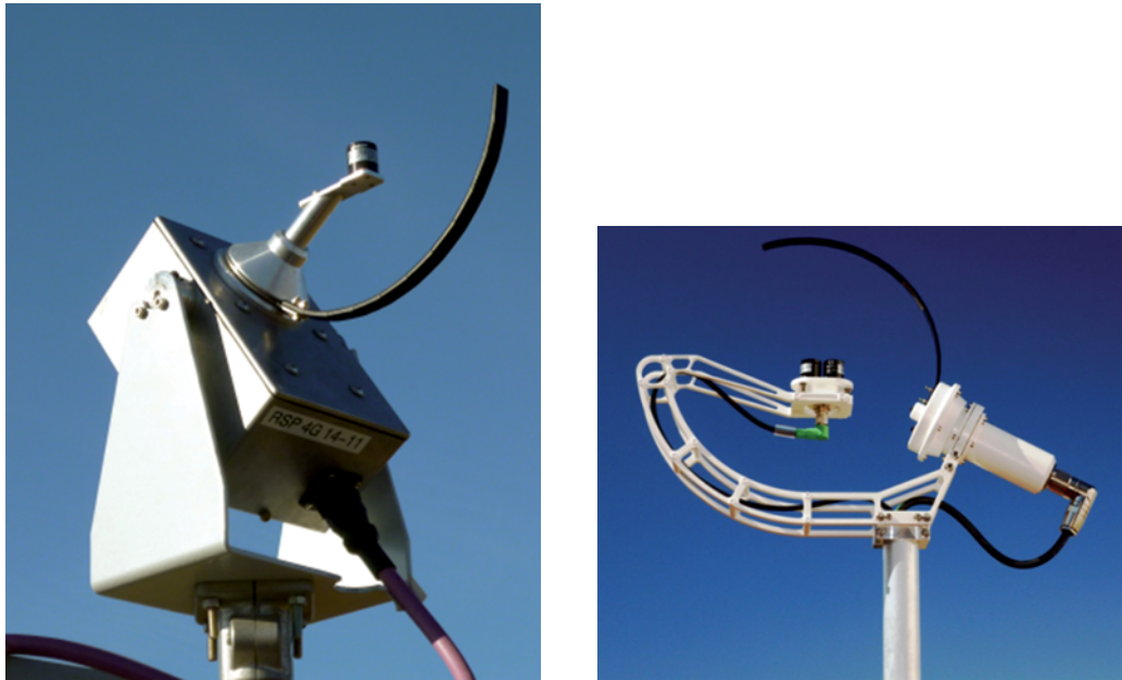
Figure 1: Left: Reichert Rotating shadowband irradiometer in rest position. Right: CSPS Twin RSI during the rotation.
