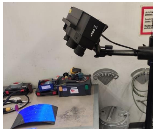
FIG. 12 Test setup for assisted scarfing process at Lufthansa Technik (Hamburg) on single curved CFRP samples [12]
