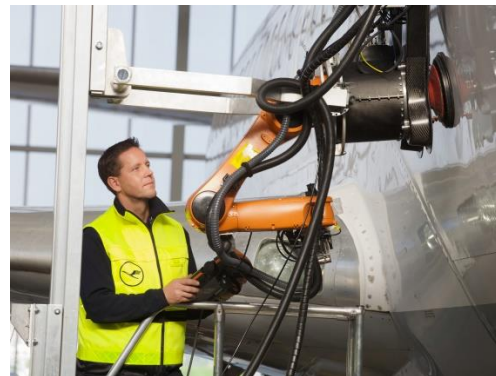
FIG. 3 Automated scarfing with CAIRE System [12]
