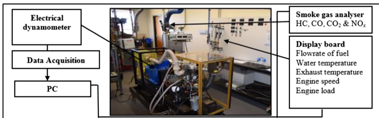
Fig. 2. Engine and control board.
