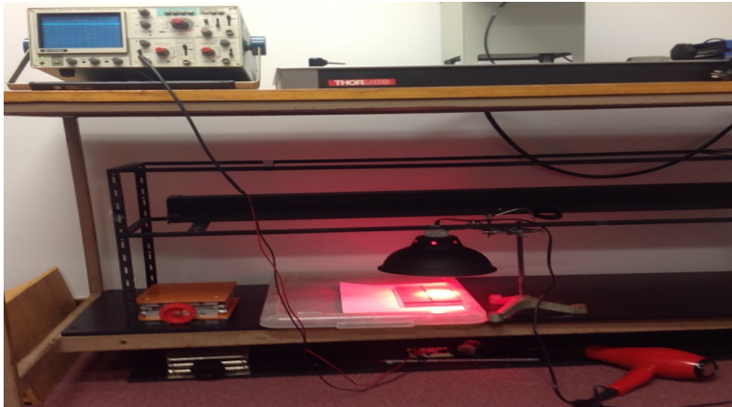
Figure 2-10: Temperature stability test setup.
