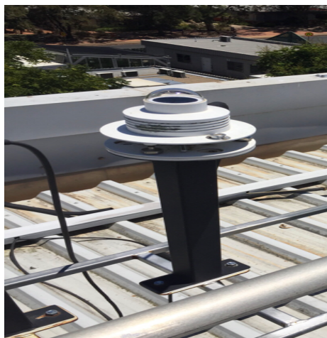
Figure 2-14: Erythemally effective five-minute exposures were monitored at the University of Southern Queensland using a broadband 501 UVB biometer (Solar Light Company PA, USA) calibrated to the erythemal action spectrum for human skin.
