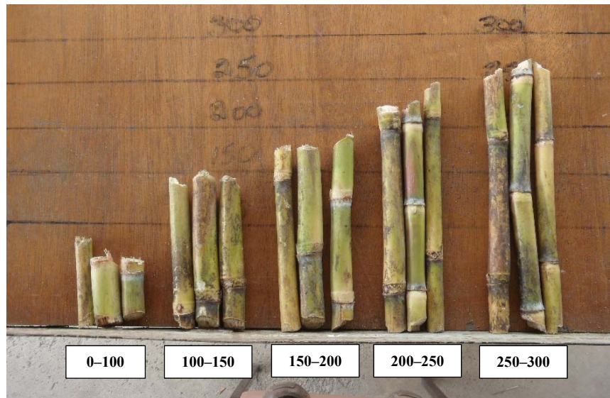
Figure 3.16 Classification of the sugarcane billet into various sizes
