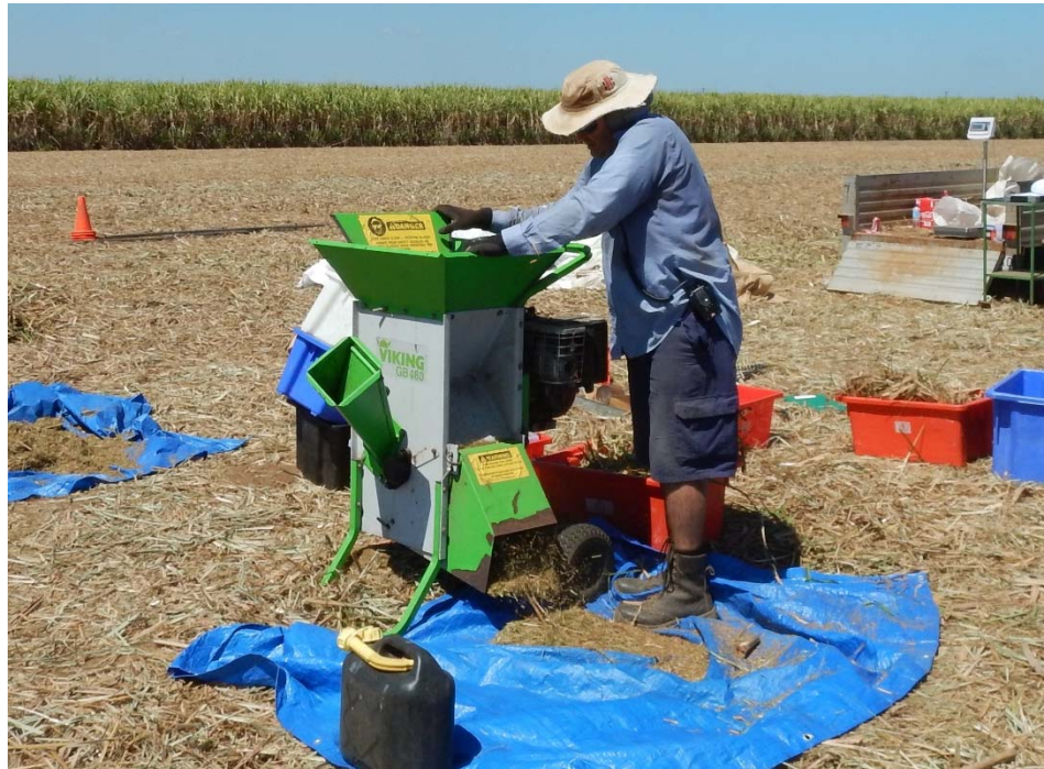
Figure 5.18 Trash was shredded using a mulcher (Viking, GB480 6 kW) (2016)
