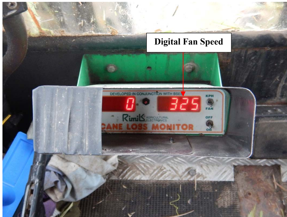
Figure 5.3 The cane loss monitor measuring the primary fan speed levels
