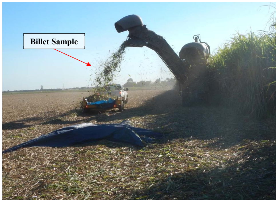
Figure 5.8 Sugarcane billet samples collected in the trailer (2016)
