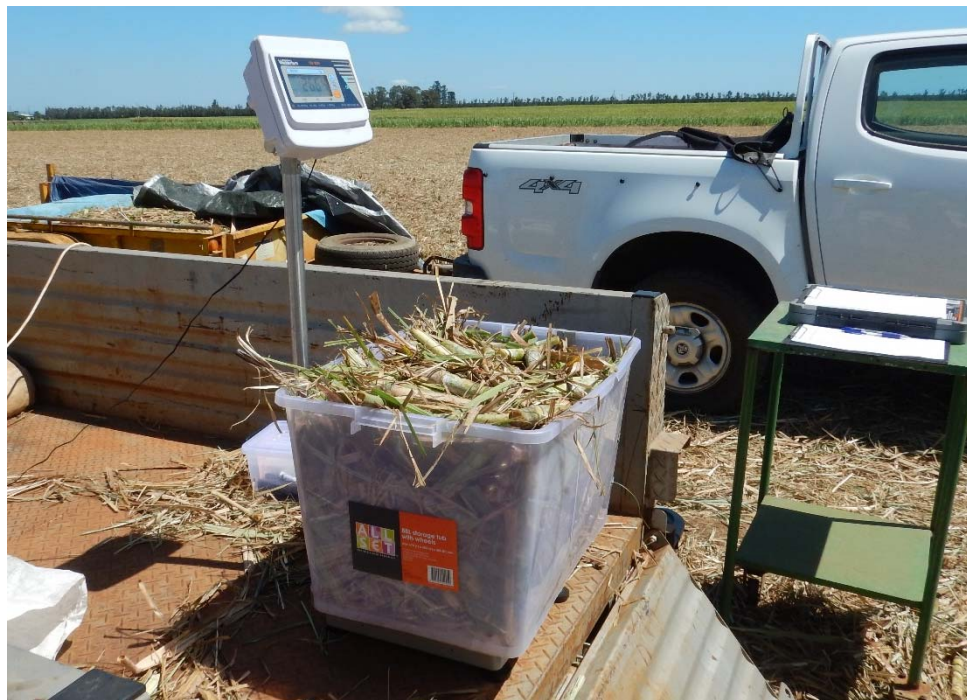
Figure 5.9 Billet sample were weighed to calculate the bulk density
