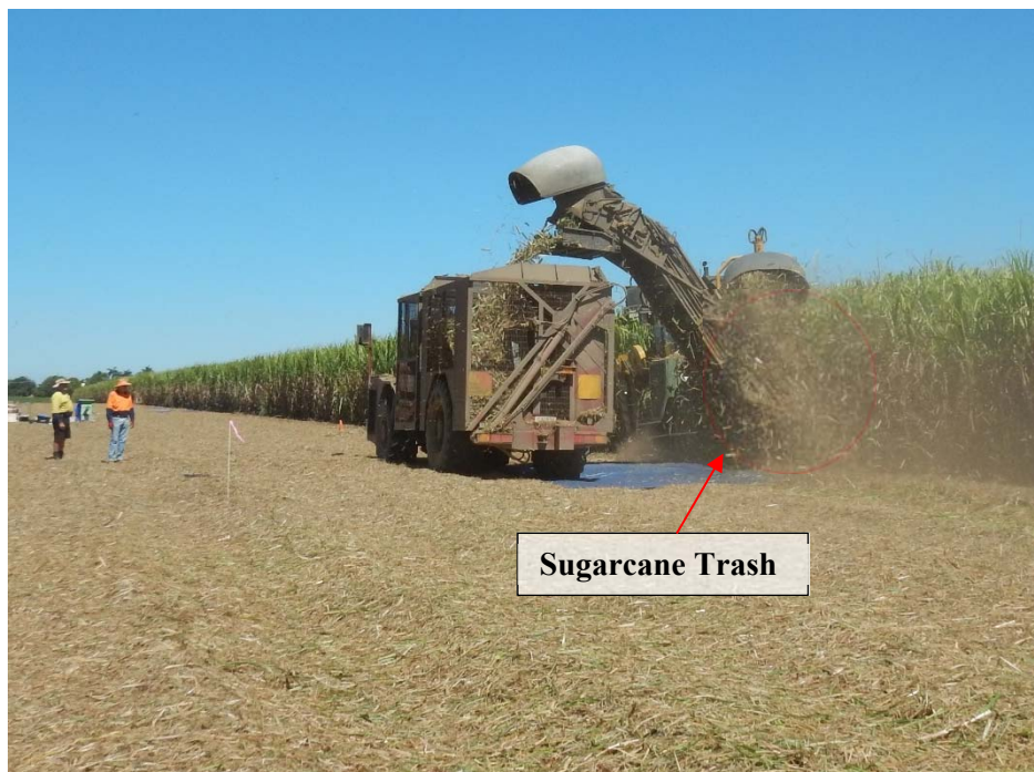
Figure 5.15 Residues blown onto the blue tarp (2016)
