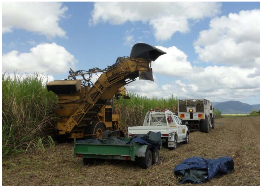
Figure 3.12 Positioning the trailer under the elevator to collect sugarcane billet samples (Ingham trial)
