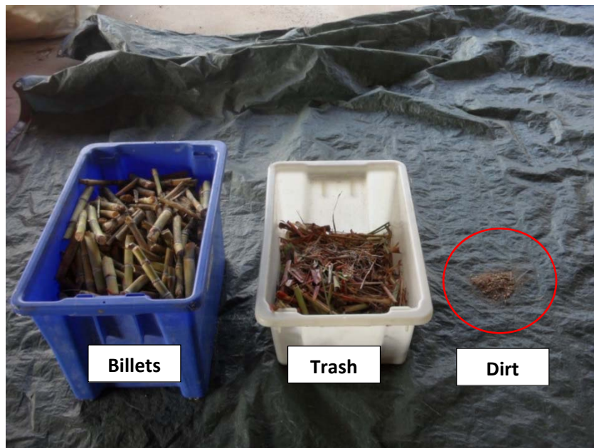
Figure 3.14 Separation of sugarcane samples into billets, trash and dirt (Ingham trial)
