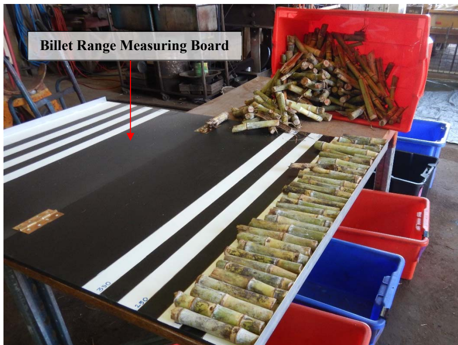
Figure 5.12 Billet length measured on a classification board (2016)
