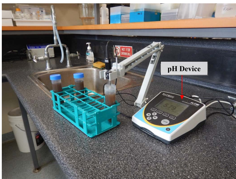
Figure 4.16 A pH meter used in the laboratory
