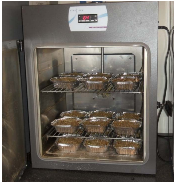
Figure 5.19 Determining the moisture content of the trash samples
