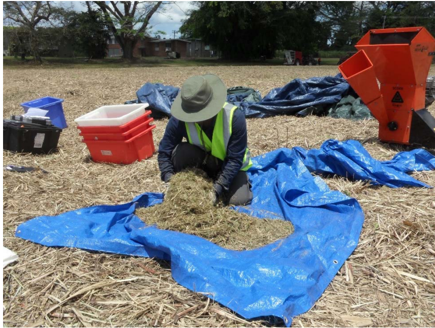
Figure 4.6 Homogenising the mulched sample (Ingham trial)
