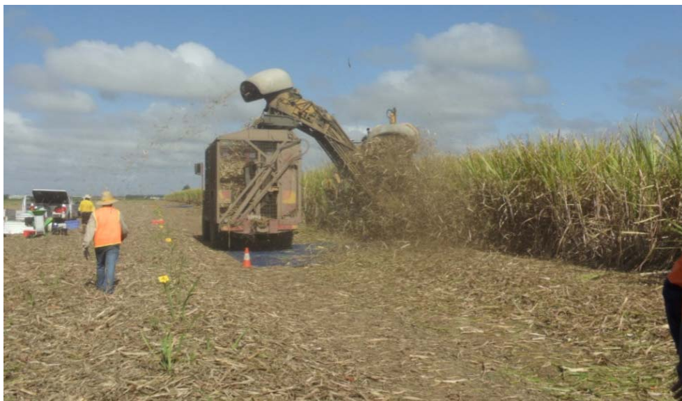
Figure 4.2 Trash is discharged from the harvester onto the blue tarps (Bundaberg trial)
