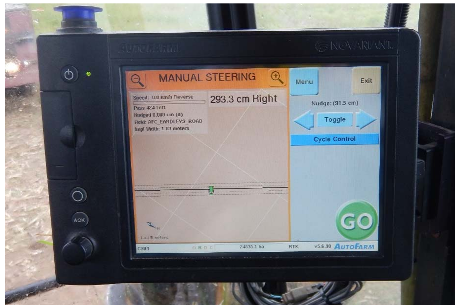
Figure 5.4 The AutoFarm monitor controlling the ground speeds during the cutting
