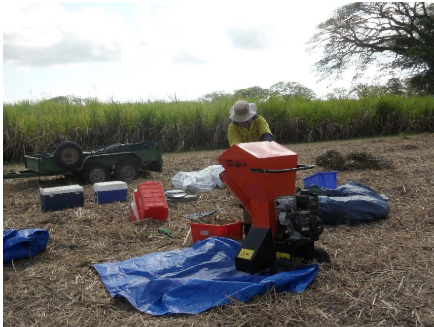
Figure 4.5 Mulching a trash sample (Ingham trial)
