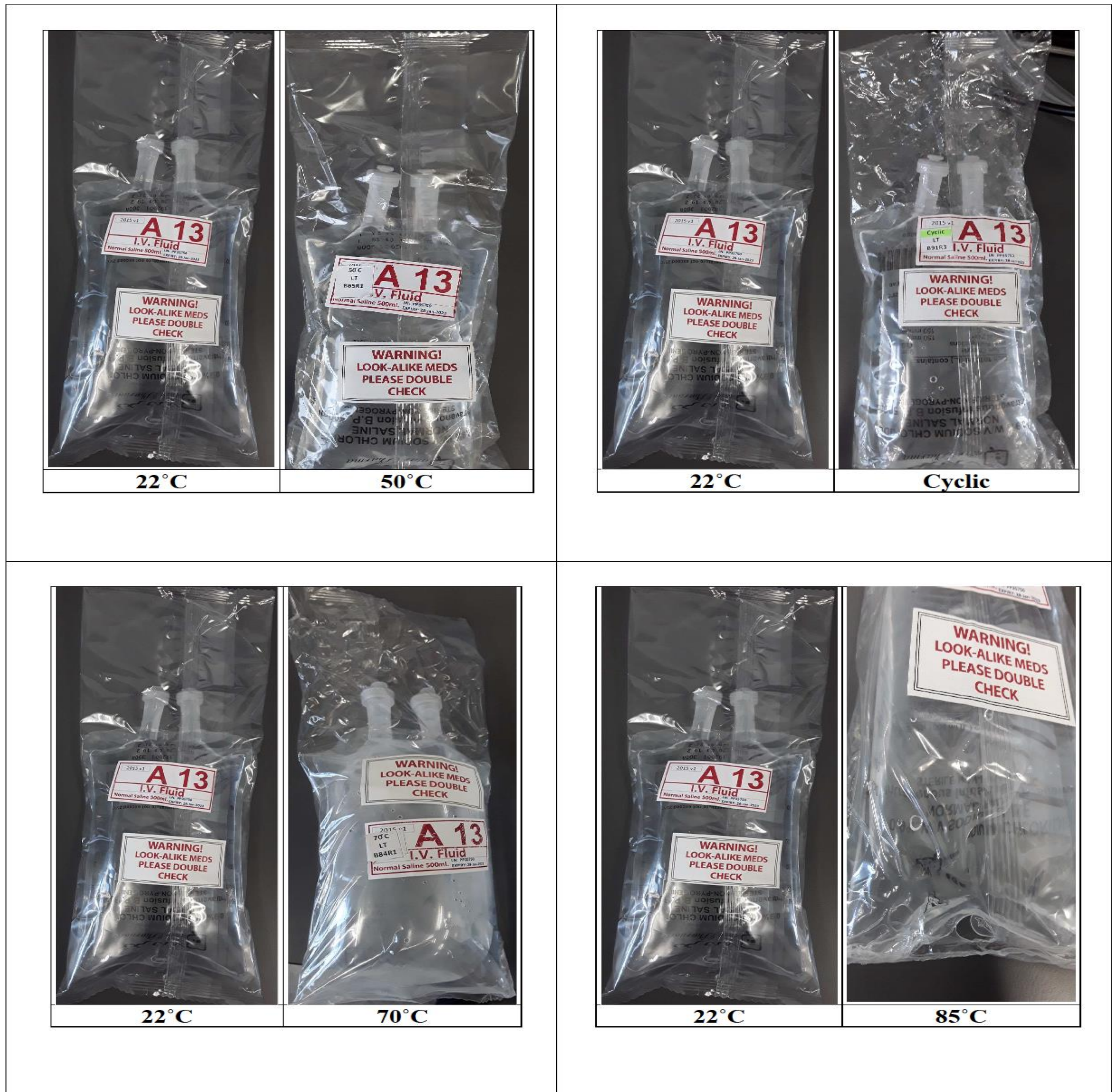
Fig. 1 Influence of temperature on bulging of normal saline container
