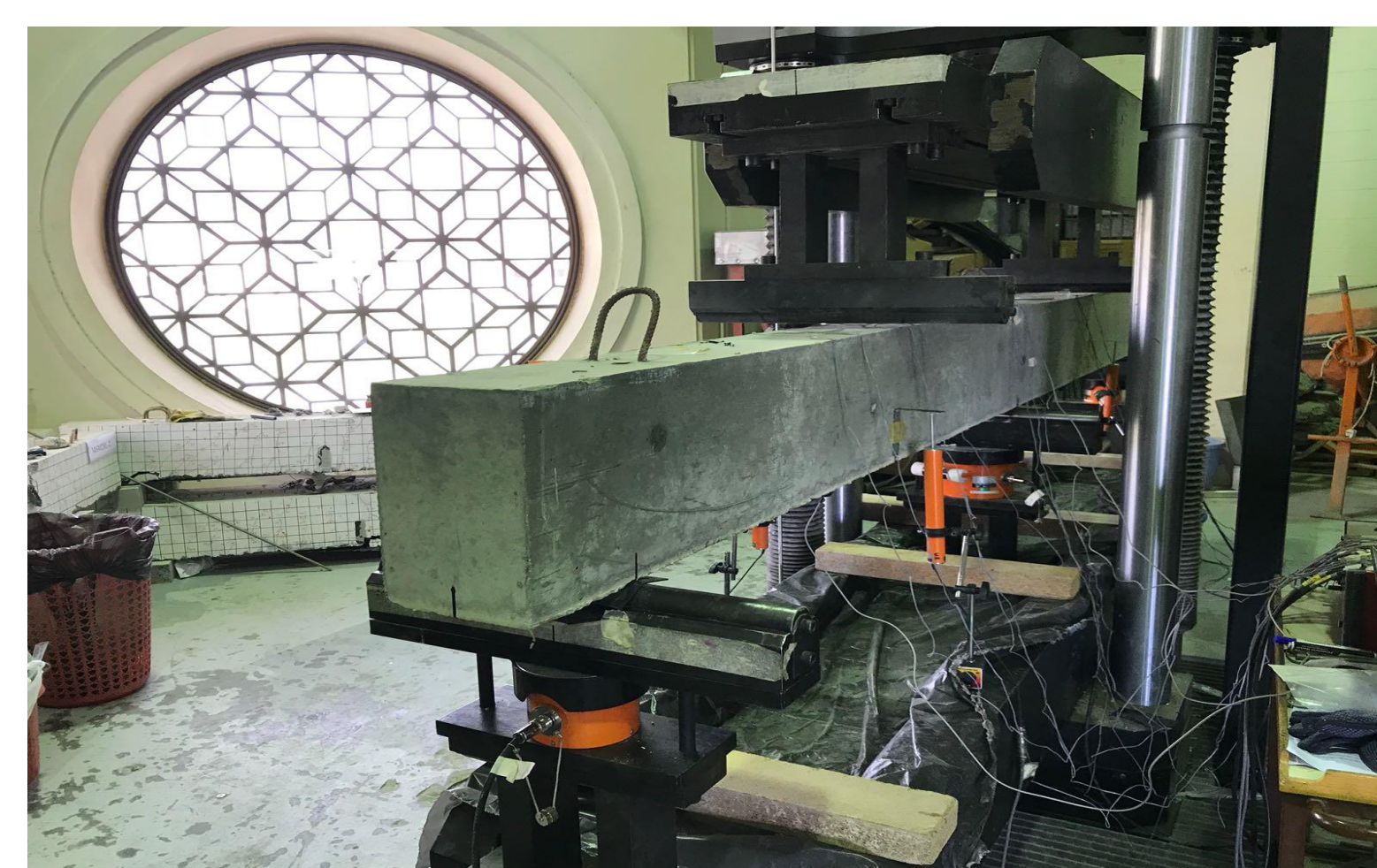
Figure 2. Experimental test setup and loading pattern
