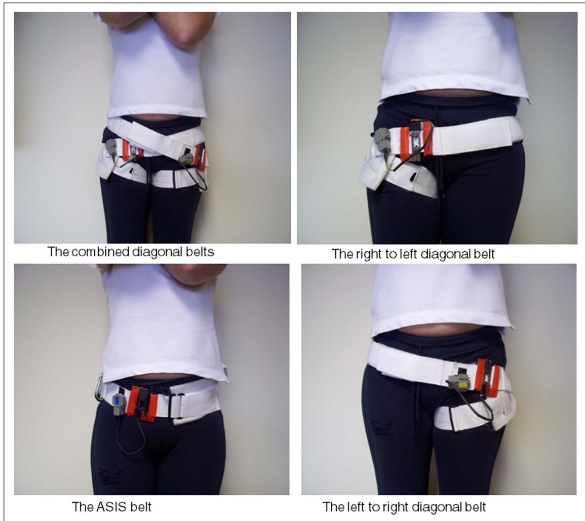
Figure 1. The pelvic belts with the strain gauges in situ.
