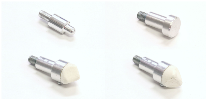
Figure 6.6: The four different indenter types used for our classification: hemispherical, flat, corner and edge tips. The edge tip (lower right) was used with orientations of 0, 120 and 240 degrees.
