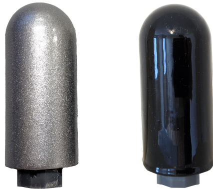
Figure 8.3: We add a black opaque layer of silicone to the DISCO Finger to remove any ambient light from leaking into the finger
