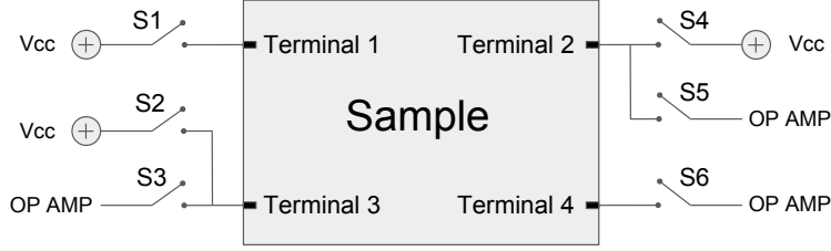
Figure 4.4: Switching Matrix structure. All six switches are controlled with digital signals from our microcontroller. This configuration allows us to measure the resistance change across any pair of terminals. The switches must be closed such that we always connect one terminal to Vcc and the remaining one to the inverting input of the operational amplifier.
