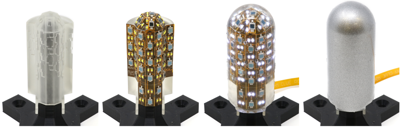
Figure 7.4: DISCO Finger through various stages of construction. We 3D-print a rigid skeleton, on which we attach a flexible circuit board with light emitters (LEDs) and receivers (photodiodes). We then mold a 7 mm thick transparent layer acting as a waveguide. Finally, we add a thin reflective outer layer.
