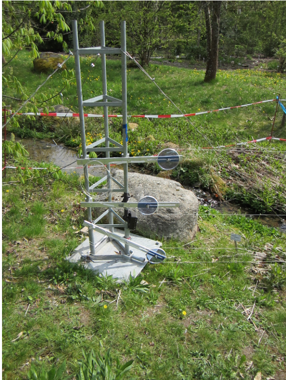
(a) Pulley-holder attached to the small tower at point A of the transect
