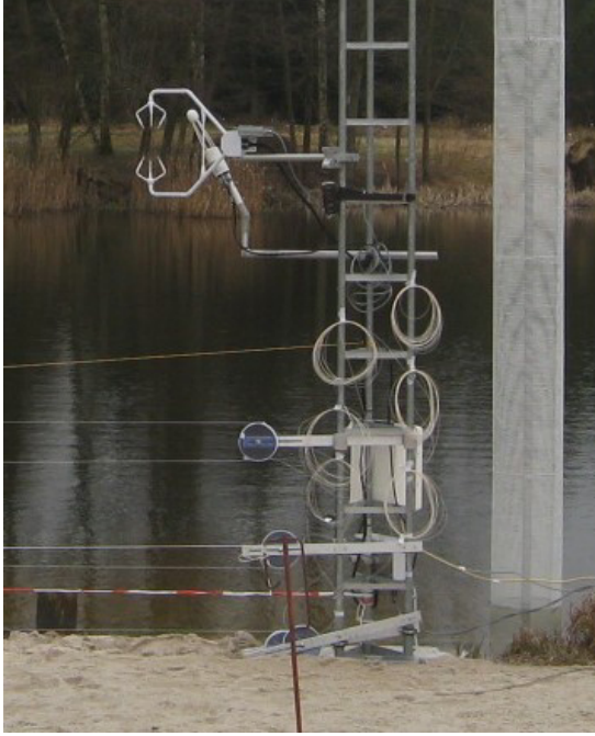
(a) first installation of CSAT and LICOR at the lake without extension of the mounting for flux measurements above the lake
