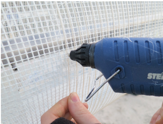
(c) Gluing fiber optic winding
