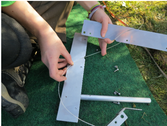
(a) Inserting the fiber into the plow
