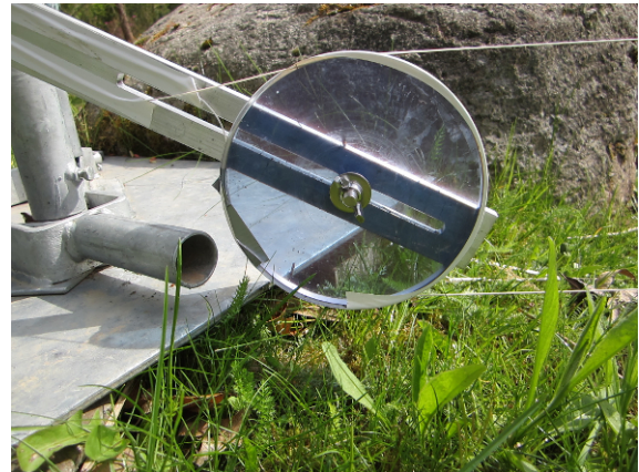
(b) Pulley-holder of 5 cm and 20 cm height at point A of the transect, close-up view
