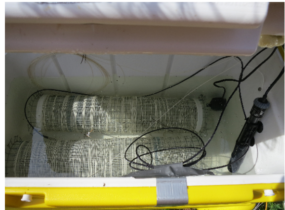
(b) Warmwaterbath with heater on the right side of the bath for 'span'-calibration
