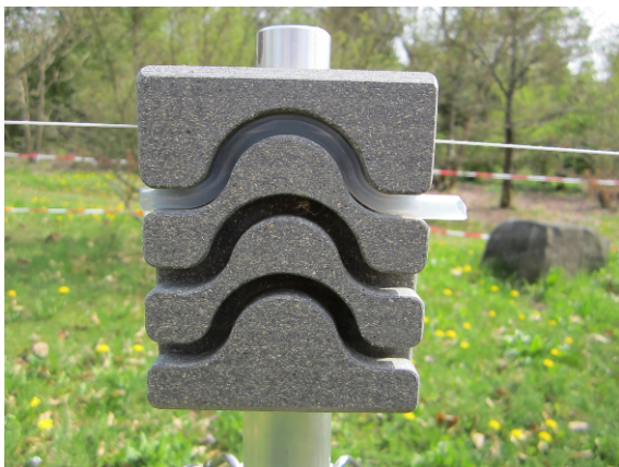
(a) Self-designed block with plastic tube
