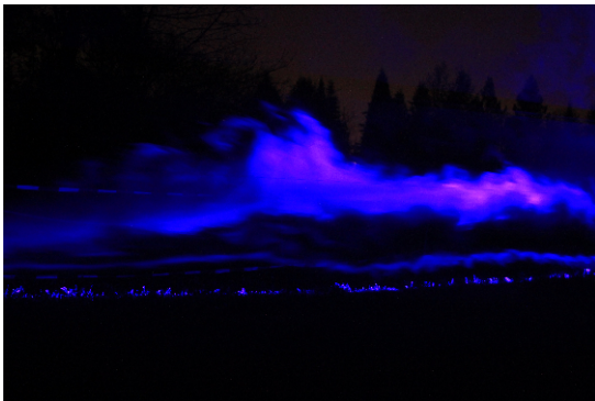
Figure 6.8 Separating flow over cold air layer without direction shear (IMG_3698.jpg)
