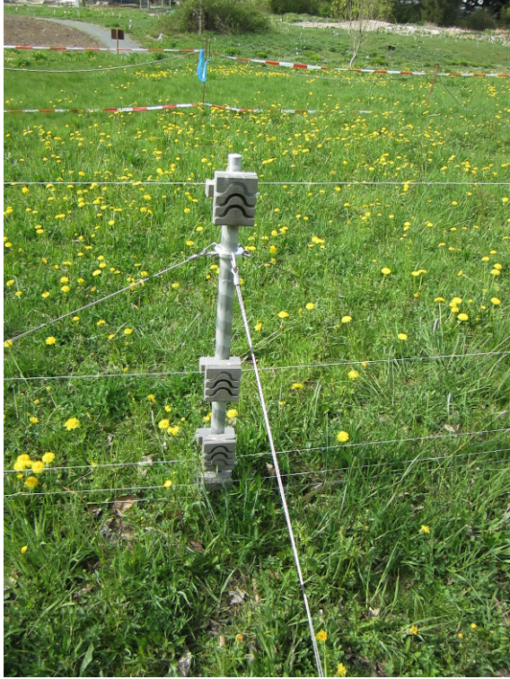
(a) self-designed poles with attached blocks and anchoring cables
