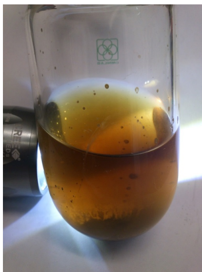
Figure S3. Photograph of the negative control after precipitation with diethyl ether.
