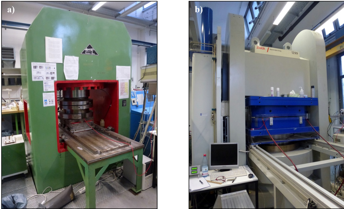
Figure 7: Multi-anvil apparatus of the Bayerisches Geoinstitut Bayreuth: a: 1000 tonne Hymag Press, b: 5000 tonne Press from Zwick and Voggenreiter.
