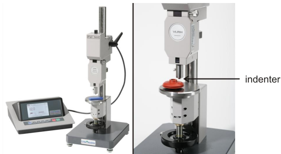
Fig. 10. left: digi test II testing device and control unit; right: VLRH measurement device with exchangeable indenter
