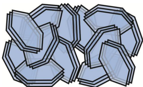
Fig. 5. House of cards structure of clay tactoids
