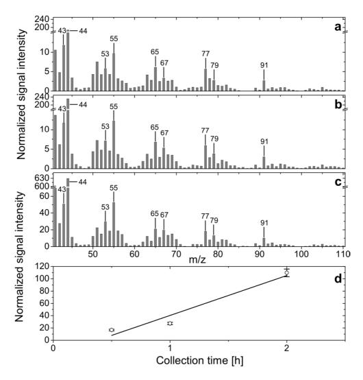
**Fig. 7:** Mass spectra of organic particles with a diameter of 25 nm from dark ozonolysis of alpha-pinene; a, b and c are spectra after collection times of 0.5 h, 1 h and 2 h, respectively. The lower panel (d) shows the sum of the signal intensities of four major peaks (m/z 55, 65, 77 and 91) in relation to the collection time.
