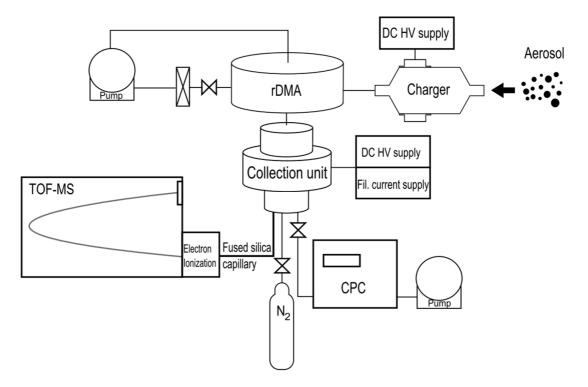
**Fig. 8:** Sketch of CAChUP, with unipolar charger, radial differential mobility analyzer (rDMA), collection unit and time of flight mass spectrometer (ToF-MS). The condensation particle counter (CPC) is located downstream of the collection unit to determine the number of collected particles. The gas phase resulting from particle desorption in the collection unit is transferred via a heated fused silica capillary to the ionization unit of the ToF-MS. Figure from Gonser and Held (2013).
