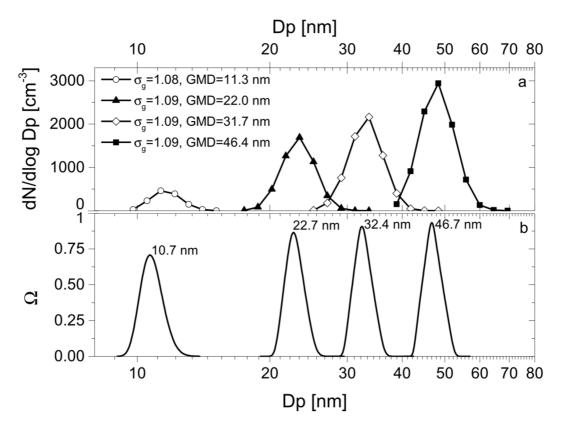
**Fig. 3:** Comparison of the performance of the rDMA coupled to an SMPS system (a) with theoretical transfer functions (b). A sheath flow of 4 SLM and voltages of 116 V, 504 V, 1003 V and 2000 V resulted in geometric mean diameters measured by an SMPS system of 11.3 nm, 22.0 nm, 31.7 nm and 46.4 nm, respectively. The theoretical transfer functions peak at 10.7 nm, 22.7 nm, 32.4 nm and 46.7 nm, respectively.
