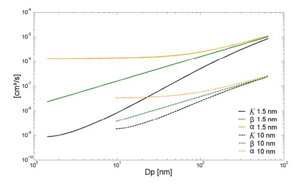
**Fig. 1:** Coagulation coefficient *K*, attachment coefficient  $\beta$  and recombination coefficient  $\alpha$  [cm<sup>3</sup> s<sup>-1</sup>] for small cluster ions and particles (1.5 nm, solid lines) and large ions and particles (10 nm, dashed lines) as function of ions and particles of diameter  $D_{p}$ .
