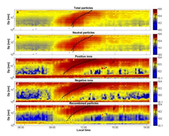
**Fig. 2:** NPF event of 12 August 2012 as measured with the NAIS. Shown are a) total particles, b) neutral particles, c) positive ions, d) negative ions and e) calculated neutral particles from ion-ion recombination. Black filled circles denote the concentration maxima for each size class, while black lines are smoothed fits in order to obtain continuous growth rates.
