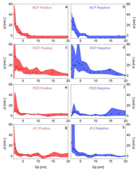
**Fig. 2**: Median values of the size dependent time difference  $\Delta t$  at Melpitz (a, b), Waldstein (c, d), Puy de Dôme (d, f) and Jungfraujoch (g, h) for positive and negative ions during all analyzed NPF events. Shaded areas represent the 25<sup>th</sup> and 75<sup>th</sup> percentile.
