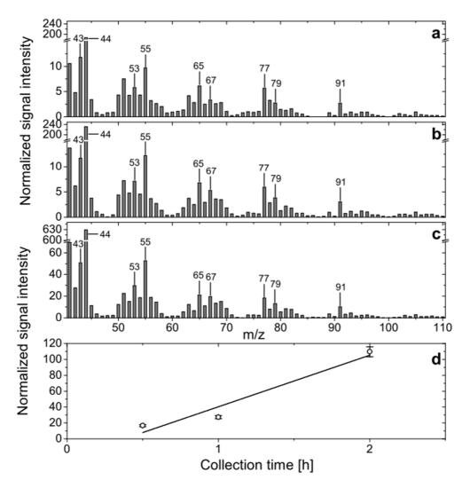
**Fig. 11:** Mass spectra of organic particles with a diameter of 25 nm from dark ozonolysis of alphapinene; (a), (b) and (c) are spectra after collection times of 0.5, 1 and 2 h, respectively. The lower panel (d) shows the sum of the signal intensities of four major peaks (m/z 55, 65, 77 and 91) in relation to the collection time. Figure from Gonser and Held (2013).
