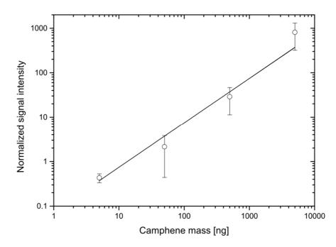
**Fig. 5:** Detection performance of the aerosol mass spectrometer for different camphene masses applied to the desorption filament. Normalized signal intensity equals the sum of the integrated peak areas of m/z 93, 121 and 136 normalized with m/z 207. Open cycles denote the mean signal intensity and the error bars show the standard deviation. A linear fit curve is shown to indicate the linearity of the signal.
