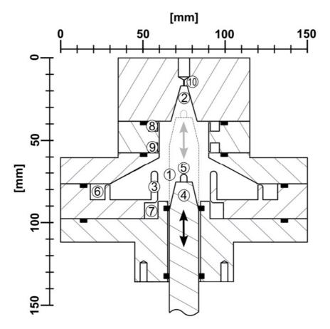
**Fig. 4:** Schematic of the radial collection and desorption unit with NiCr filament in collection position: (1) collection region, (2) desorption region, (3) collection tube, (4) PEEK piston, (5) collection filament, (6) aerosol inlet, (7) collection flushing inlet, (8) desorption flushing inlet (9), exhaust and (10) screw connection for transfer capillary. Positions of O-rings are shown in black.
