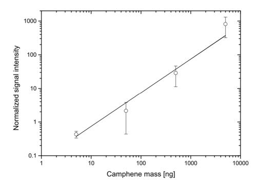
**Fig. 10:** Detection performance of CAChUP for different camphene masses applied to the desorption filament. Normalized signal intensity equals the sum of the integrated peak areas of m/z 93, 121 and 136 normalized with m/z 207 (for further detail see Gonser and Held (2013)). Open cycles denote the mean signal intensity and the error bars show the standard deviation. A linear fit curve is shown to indicate the near to linear behavior of the signal. Figure from Gonser and Held (2013).
