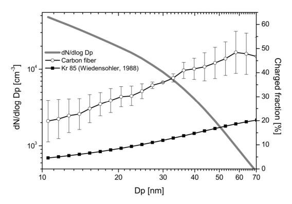
**Fig. 2:** Size dependent extrinsic charging efficiency of the unipolar carbon fiber corona charger, and the theoretical charging efficiency of the bipolar charge equilibrium (Wiedensohler, 1988) for singly positive charged particles. Additionally, the number size distribution of the aerosol used for characterization is shown.
