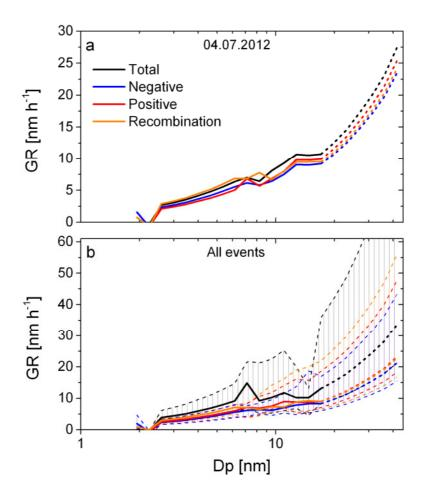
**Fig. 6:** Growth rates of negative ions, positive ions and total particles determined from NAIS measurements, a) for a single event on 04 July, 2012 and b) median values for all 8 selected NPF events used for this study. Hatched areas denote the  $25^{th}$  and  $75^{th}$  percentile. Additionally, GR<sub>rec</sub> deduced from ion-ion recombination is shown in orange. Dashed segments of the curves denote inaccurate growth rates.
