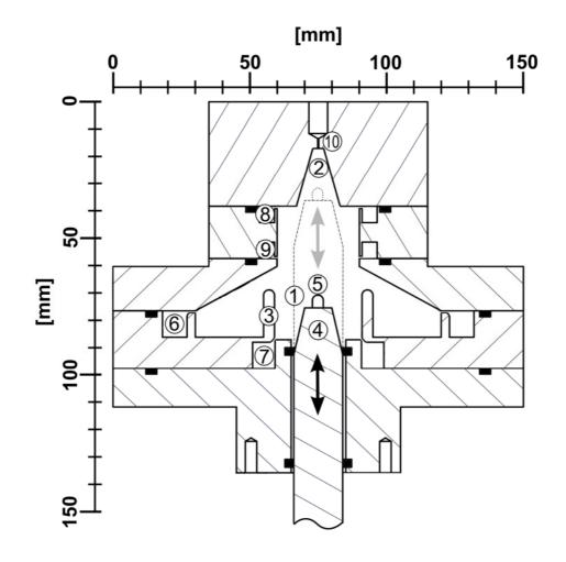
**Fig. 9**: Schematic of the radial collection and desorption unit with NiCr filament in collection position: (1) collection region, (2) desorption region, (3) collection tube, (4) PEEK piston, (5) collection filament, (6) aerosol inlet, (7) collection flushing inlet, (8) desorption flushing inlet, (9) exhaust and (10) screw connection for transfer capillary. Positions of O-rings are shown in black. Figure from Gonser and Held (2013).
