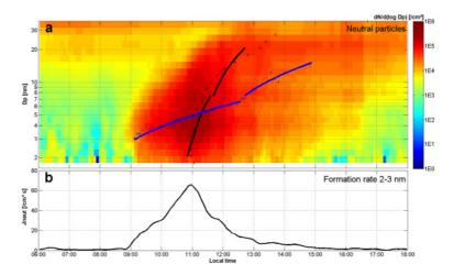
**Fig. 5**: NPF event on 31 August, 2008 at Melpitz measured with the NAIS. Shown are (a) neutral particles and the results of two GR methods. Blue crosses and lines represent results from the mode fitting method, black lines and crosses represent results from the maximum concentration method. Panel (b) shows the progression of the neutral particle formation rate in the diameter range 2-3 nm.
