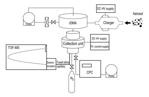
**Fig. 1:** Sketch of the instrument setup, with particle charging unit, radial differential mobility analyzer (rDMA), collection and desorption unit and electron ionization time of flight mass spectrometer (TOF-MS).
