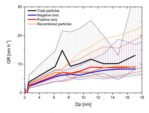
**Fig. 5**: Median growth rates of negative ions, positive ions, total particles and recombined neutral particles determined from NAIS measurements of 8 selected NPF events at WST during summer 2012. Hatched areas denote the 25<sup>th</sup> and 75<sup>th</sup> percentile. Figure adapted from Gonser et al. (2014a).
