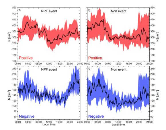
**Fig. 3:** Median diurnal variation of cluster ion concentrations (diameter < 1.6 nm) during 8 selected NPF event days (a, c) and 13 non-event days (b, d), as measured with the NAIS during summer 2012 at the "Waldstein" site. The shaded areas denote the 25<sup>th</sup> and 75<sup>th</sup> percentile.
