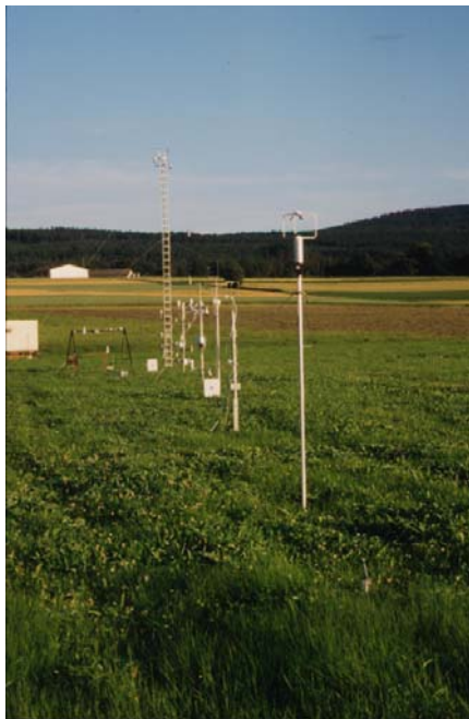
Fig. 1: Sonic anemometers during the VOITEX-99 experiment: In the foreground Young No. 81000 followed by Gill Instruments 'Solent R2', two METEK 'USA-1' and 'CSAT3'.
