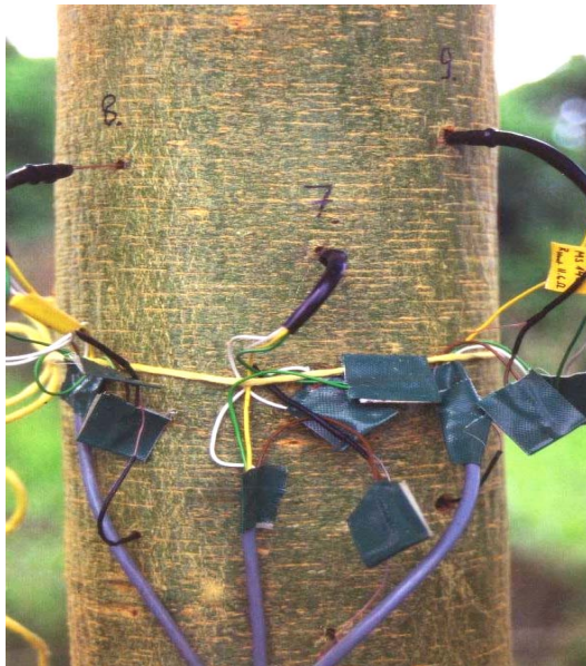
Plate 1. Three sap flow sensors numbered 7, 8 and 9, installed at different depths (0-20, 20-40 40-60 mm respectively) into the trunk of A. xanthophloea .
