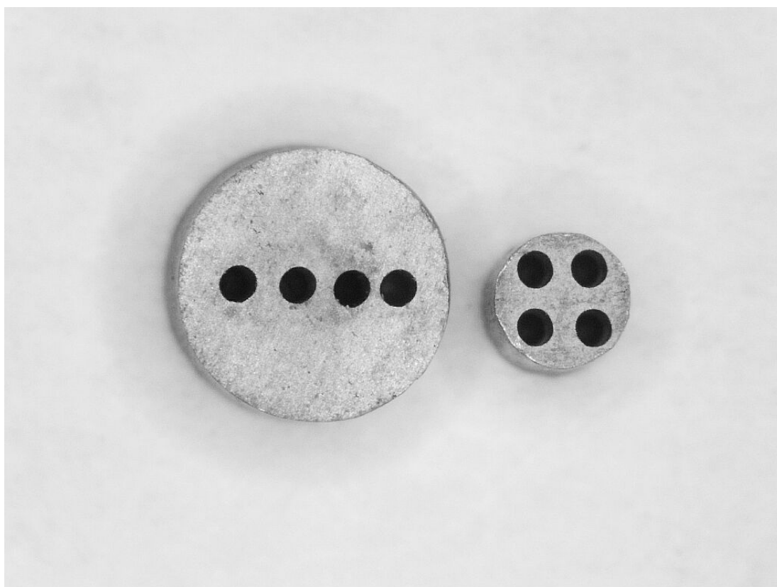
Figure 2.3: Examples of Re multi-chamber capsules produced by spark-erosion. Diameters of the capsules are 2 and 1 mm, respectively. Capsule heights were usually close to 1 mm. Sample chambers are approximately 250\ \mu\text{m} in diameter. The left capsule can be used in the 18/8 assembly up to 24 GPa, while the smaller 1 mm capsule can be used up to 26 GPa using 10/4 or 8/3 pressure cells. Due to relatively small thermal gradients in pressure cells with stepped furnaces (18/11, 18/8) up to two multi-chamber capsules could be used in a single experiment.
