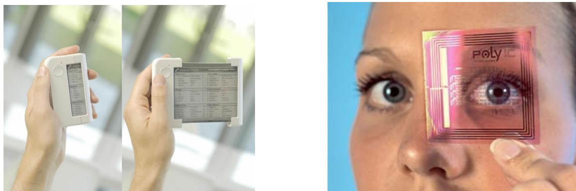
Figure 1-3. E-reader with rollable display and Q-VGA resolution from Philips (left) and a design study of an organic RFID tag, prepared by roll-to-roll printing technique from PolyIC (right, www.polyic.com ).
