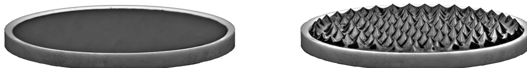
Figure 1.3: The experimental realization of the Rosensweig instability. On the left hand side the applied magnetic field (applied normal to the surface) is below the critical value whereas the picture on the right hand side is taken beyond the critical value. The containers diameter is of the order of 20 cm and the height as well as the diameter of the spikes is in the order of 1 cm.
