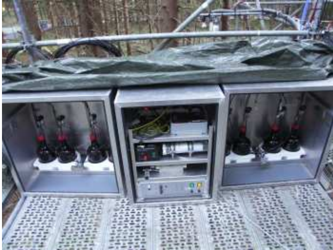
Sub-canopy CO 2 measuring system
