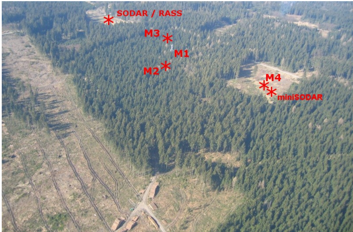
Fig. 2: Actual state of the measuring sites and positions of the main tower M1, turbulence tower M2, bio tower M3, modified Bowen ratio mast M4, SODAR / RASS, and miniSODAR systems.
