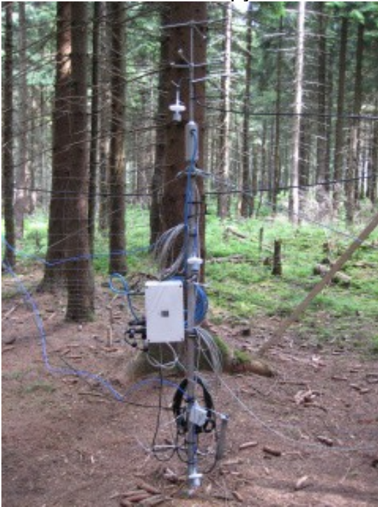
Advection sub canopy mast M10
