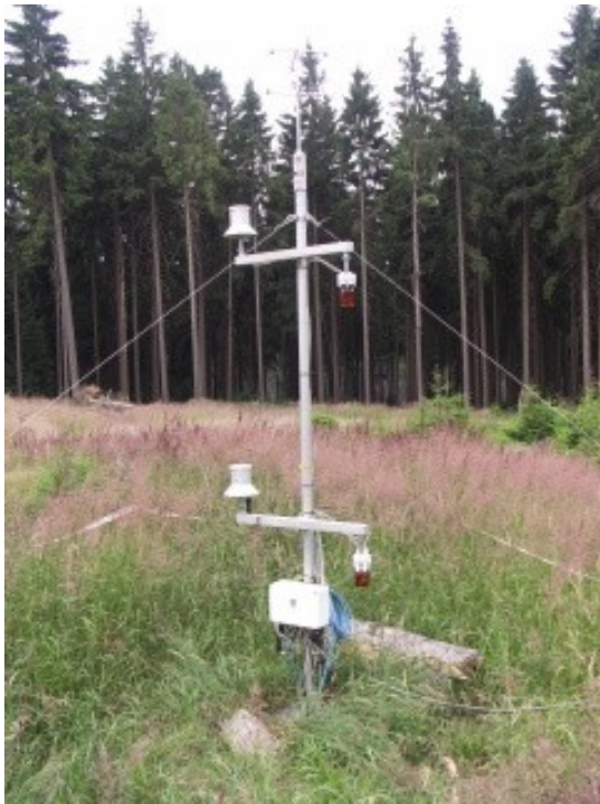
Modified Bowen ratio mast
