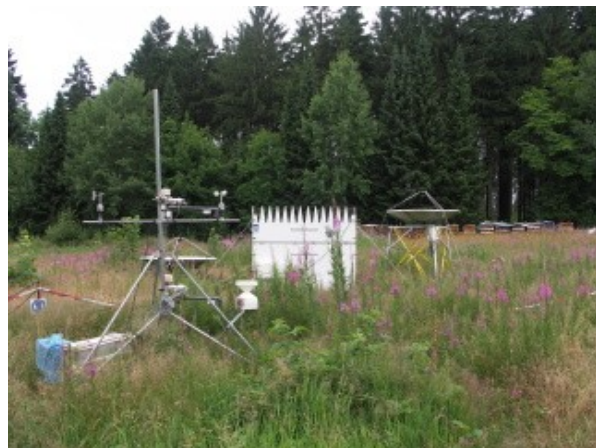
SODAR/RASS and weather station
