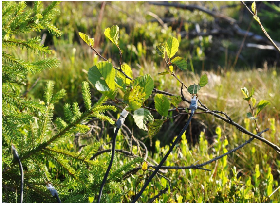
Leaf wetness sensors (leaf clamps) on alder (left) and on grass (right)
