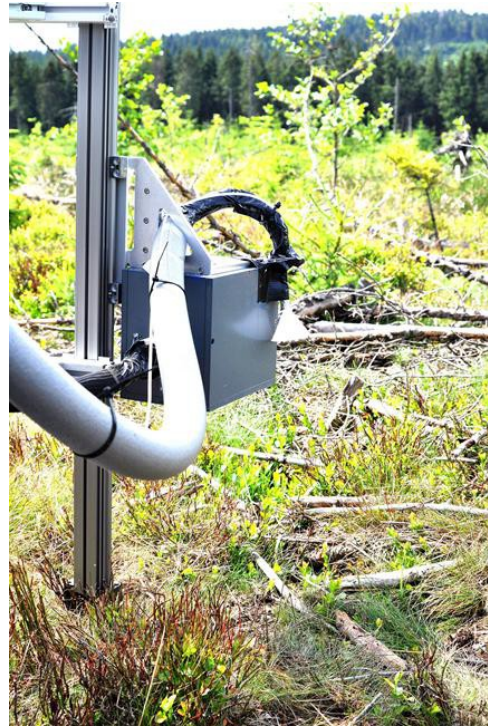
Structure with the LOPAP instrument and the elevator (detail of the movable inlet on the right side)
