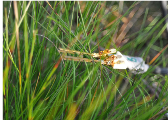
Leaf wetness sensors (leaf clamps) on alder (left) and on grass (right)
