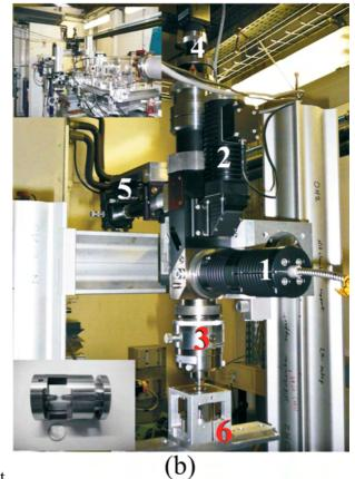
SPI100 fibre laser; **2**, illumination unit; **3**, lenses unit for focusing of the incoming laser light; **4**, digital video camera; **5**, module for spectroscopic measurements; **6**, DAC mounted inside the holder; **7**, mounting plate; **8**, holder for a carbon laser mirror.
