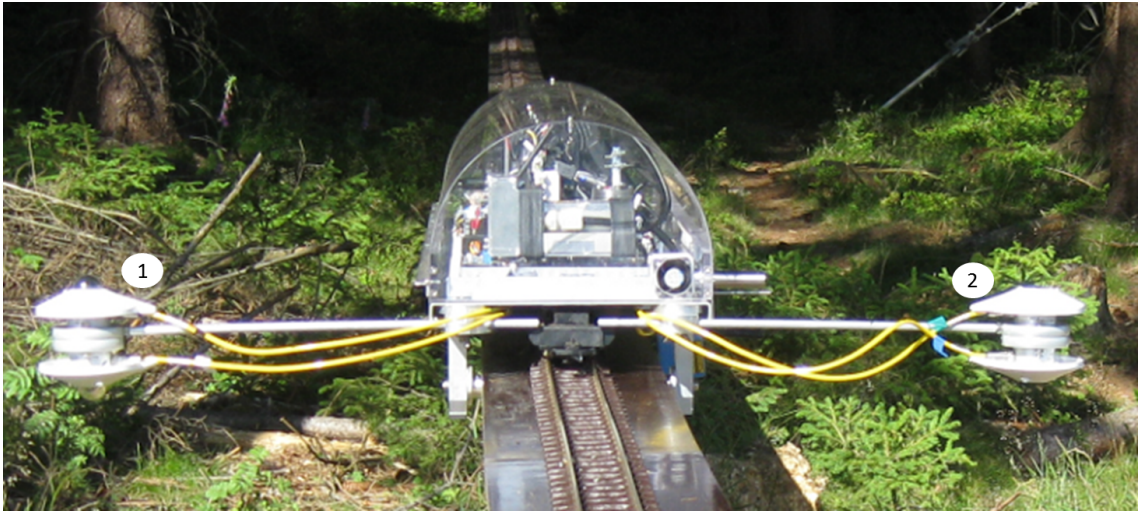
Figure 4.3: Front view on the HMMS. In forward direction the two short-wave radiation sensors Kipp & Zonen CMP3 are located on the right side ①. And on the left side the two long-wave radiation sensors Kipp & Zonen CGR3 ②.
