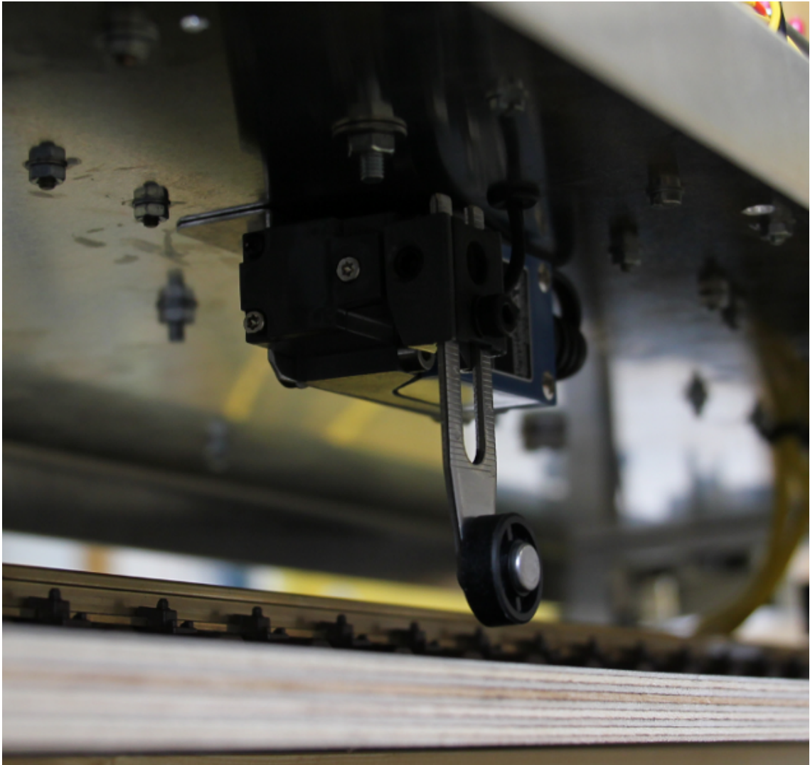
Figure 2.5: Moving limit switch mounted bottom side at the base plate of the HMMS. The moving limit switch can be thrown in both directions and cut off immediately the power supply to the engines.
