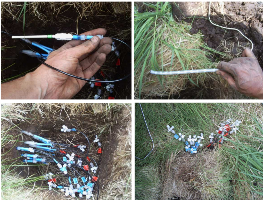
Figure 2. Installation of soil gas and pore water samplers in a peat profile.
