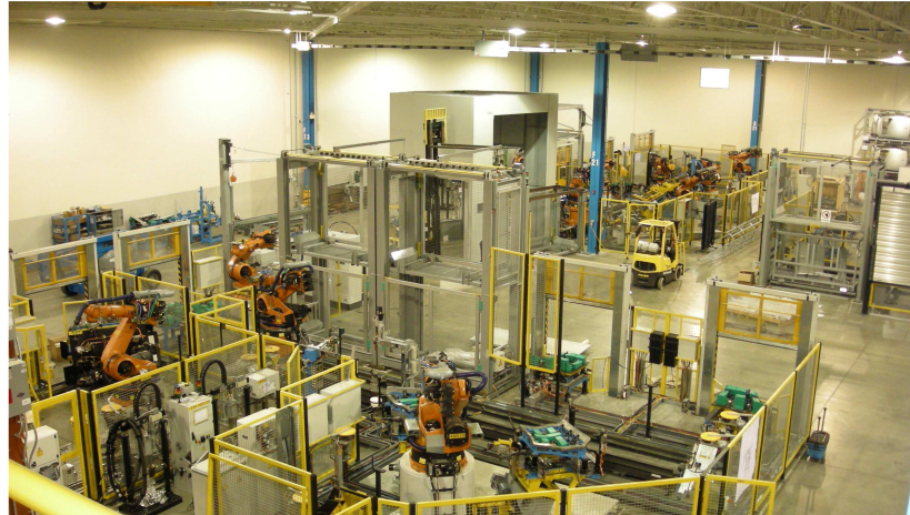
Figure 1.5: Industrial robots separated from humans by fences [129]
