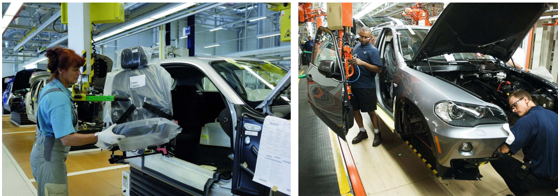
Figure 1.6: CoBots. Left: Seat assembly [34]. Right: Door assembly [33]
