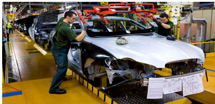
Figure 5.2: The assembly line workers are fixing the wind screen on a vehicle. The wind screen is carried by a device and guided to its exact location by the human workers [72]. In case of intuitive HRI the robot can create ease of navigation by slowly moving in the guided direction and proactively cooperating in the next tasks
