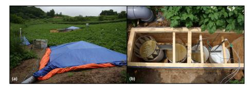
Figure 1.3 Runoff sampler for measuring runoff volume and sediment mass according to Bonilla *et al.* (2006). Runoff collectors (a) and multislot flow divider according to Pinson *et al.* (2004) (b)
