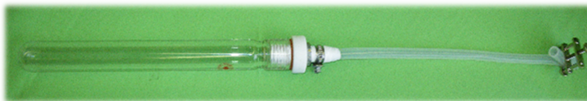
Figure 1. Reaction flask closed with a silicone tube ((Rotilabo®) inner diameter 7 mm, outer diameter 10 mm and 30 cm length) as semi-permeable membrane was used for the pyridine syntheses.
