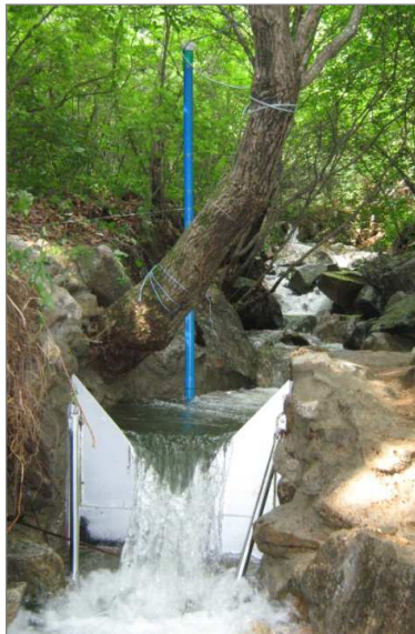
Figure 1.2: Sharp-crested V-notch weir located at the forested head water site S1.
