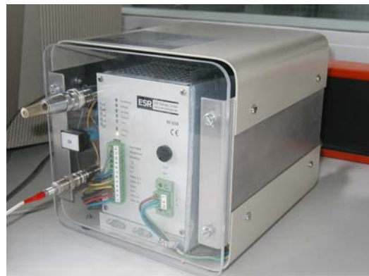
Figure 4.16: Power amplifier for the DC motor
