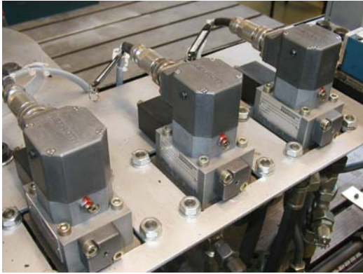
Figure 4.17: The three servo valves
