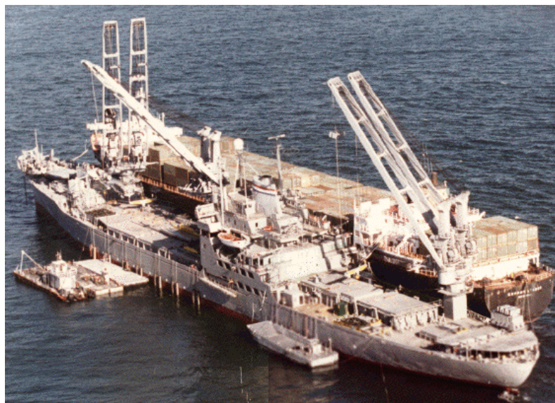
Figure 1.1: Picture of a ship-mounted crane at sea
