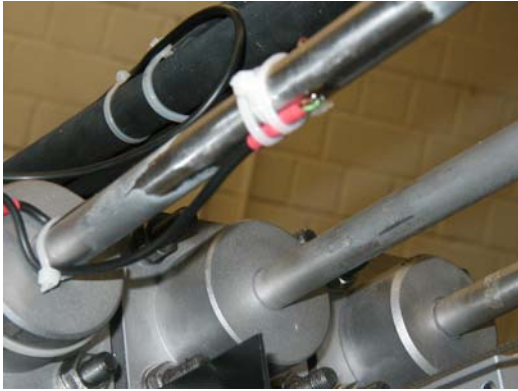
Figure 4.10: Strain gauge for measuring the elastic rotational displacement
