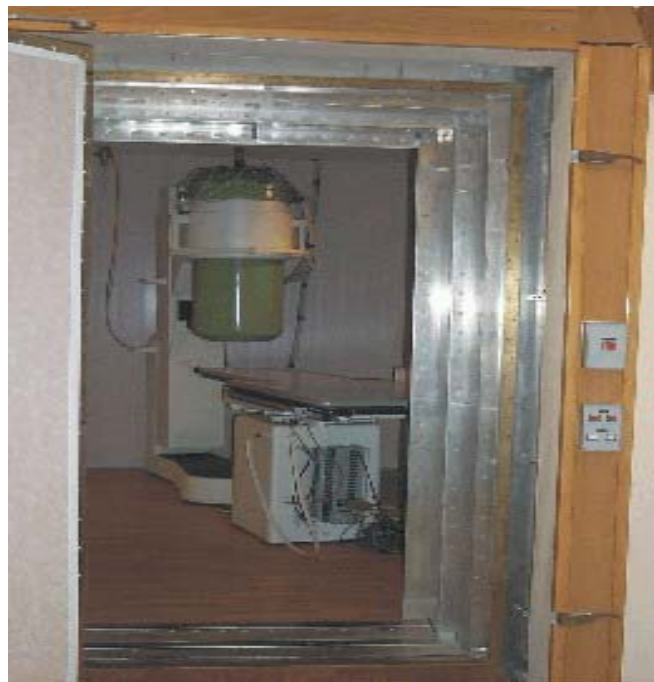
Figure 2: Multi-channel MCG system (Phillips) installed in the shielded room
