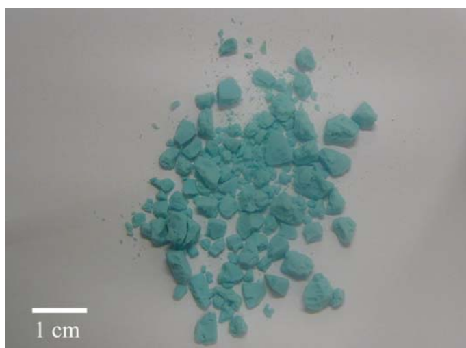
Fig. 7-17: Photograph of the Cu-Al dried aerogel (Cu:Al = 1:1), dried in supercritical CO 2 .
