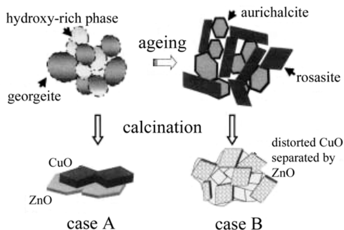
Fig. 2-7: Evolution of the microstructural characteristics with ageing of the precursors and the resulting oxides 41 .
