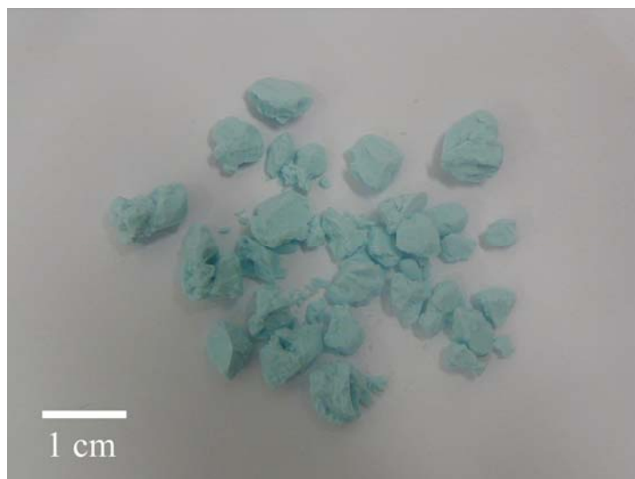
Fig. 7-21: Photograph of the Cu-Zn-Al dried aerogel (Cu:Zn:Al = 1:1:1).
