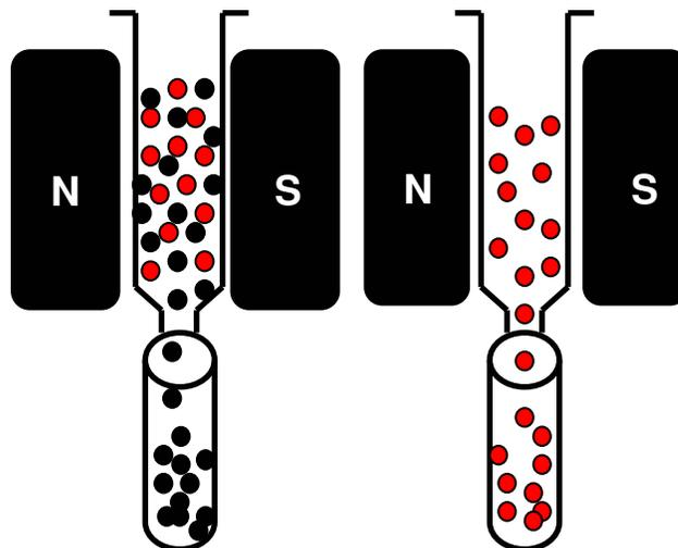
**Figure 7:** Magnetic cell separation using autoMACS. Labeled cells (shown in red) are retained in the column while unlabeled cells (shown in black) are collected as flow through. On further washing with MACS buffer and under controlled pressure, the retained fraction can be eluted.
