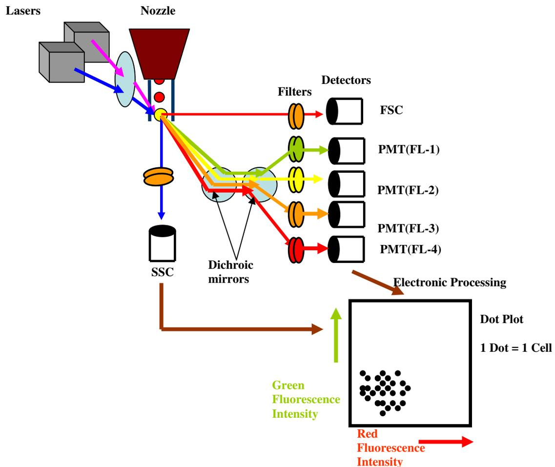
**Figure 8:** Schematic overview of a typical flow cytometer setup and the principle of flow cytometry.
