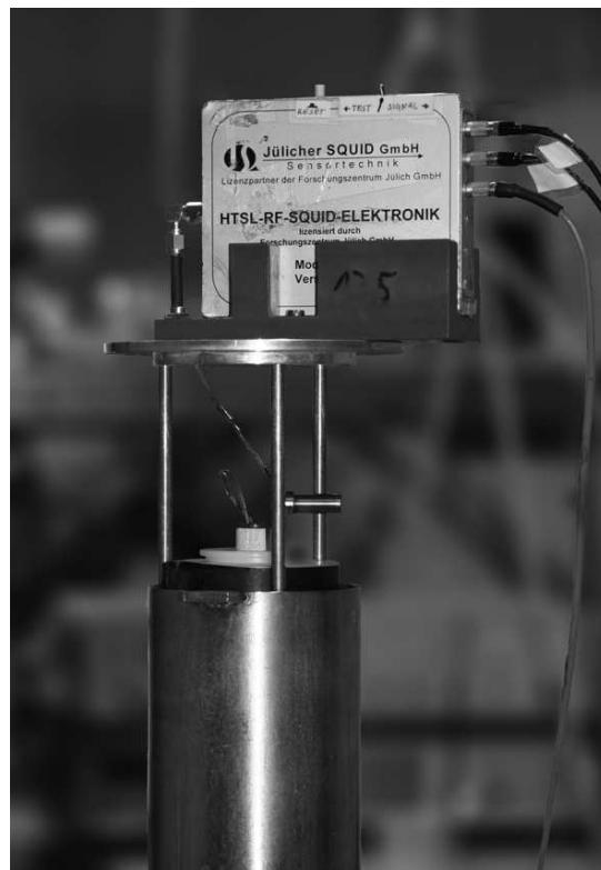
Fig. 3.11.: SQUID electronics and the electrical shielding, which has been lowered for the photograph.
