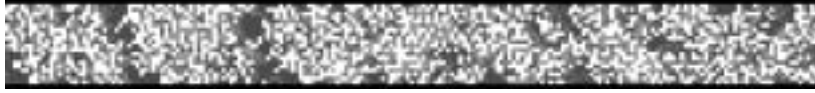
Fig. 3.6. Density for a square lattice with periodic boundary conditions and global density \rho = 4.4 \text{ P/m}^2 . The occupied cells are indicated by dark, the empty by white dots. Jam waves moving opposite to the walking direction, which is from left to right, can be observed.
