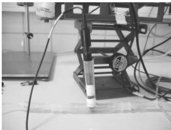
Figure 2.1: Flow cells used in combination with electrodes for effluent or influent online measurement.
