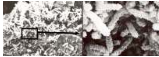
Figure 1.7: Iron oxides precipitated on bacteria in corrosion products of a drinking water pipe (from Flemming and Leis, 2002, modified).
