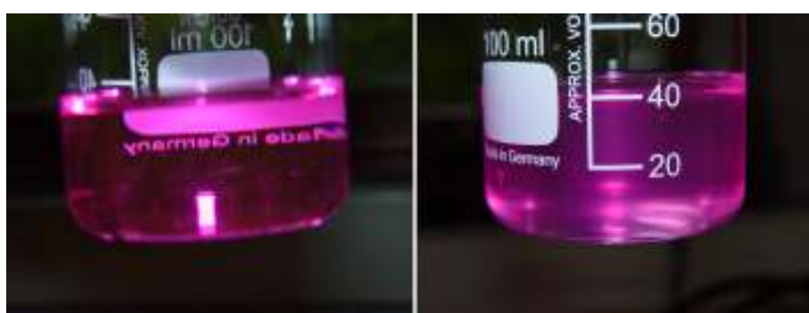
Figure 3.11: Right: 2000 mg L -1 LRD+R6G suspended in 70 mM NaCl before dialysis. Left: same suspension after dialysis. No rhodamine outside the dialysis tube, no decrease in rhodamine 6G spectrophotometric signal were found.
