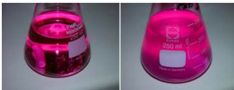
Figure 3.10: Aggregation process of rhodamine 6G-stained laponite RD. Left: 2000 mg L -1 stained laponite RD suspended in deionized water. Right: same suspension in 70 mM NaCl.
