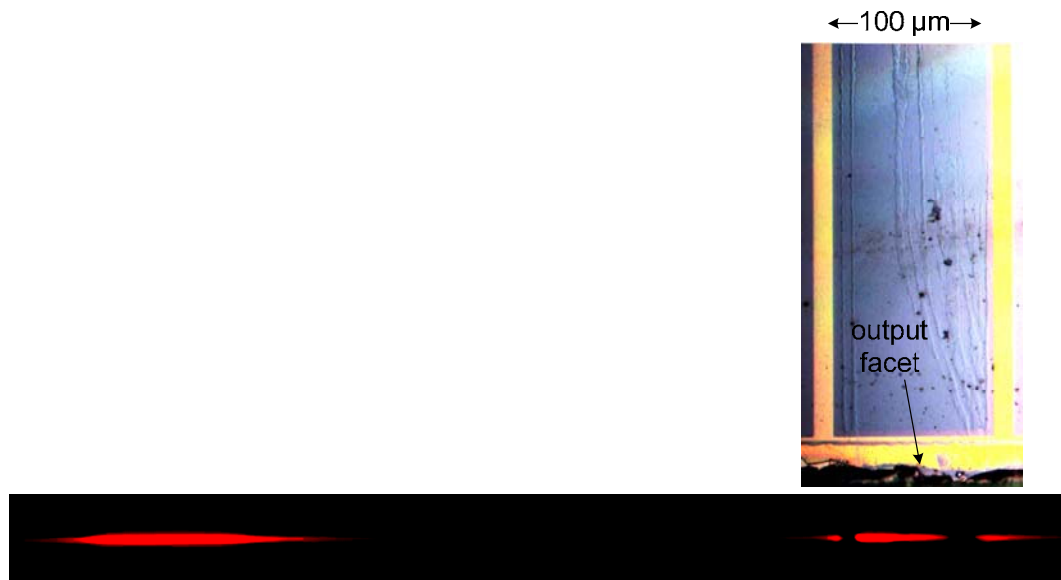
Fig. 4.2.13. 10-Emitter high-power laser bar with pulsed COD (pulse width: 1 \mu s, pulse frequency 10 kHz). Right: the laser that had a COD and its corresponding EL is shown. Left: the EL of the neighboring laser where no COD occurred.
