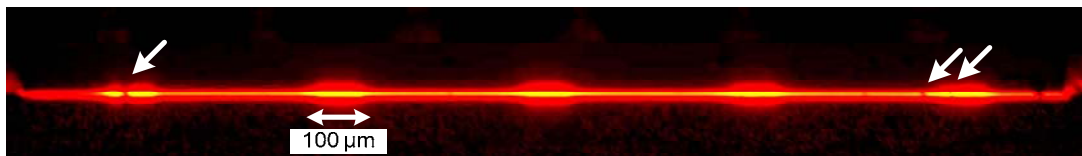
Fig. 4.2.11. EL of a 635 nm 5-emitter high-power laser bar where the side lasers underwent a COD event (dark spots are pointed by arrows).
