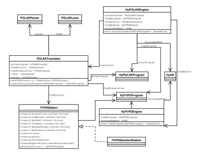
Figure 6.1: POLAR translation and execution classes as UML class diagram
