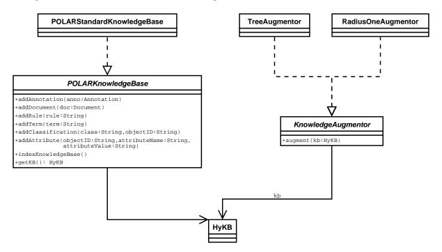
Figure 6.2: POLAR indexing classes as UML class diagram
