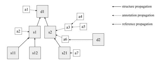
Figure 4.4: Annotation-based structured document retrieval. Grey boxes reflect subparts of a structured document, white boxes are annotations. Arrows denote structure, annotation and reference propagation, respectively.
