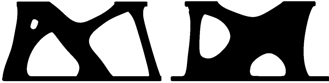
Fig. 5.21: For comparison, we also ran Algorithm 4.11 using the barrier approach for the same configuration shown in Fig. 5.20 with \eta = 0.4 . The left picture shows the result with s = 0.8 in Algorithm 4.5, whereas the right picture was obtained with s = 0.9 . The objective value, i.e. the value of the objective function of problem (3.39), for the left shape was 0.00395, and for the right shape 0.00808.
