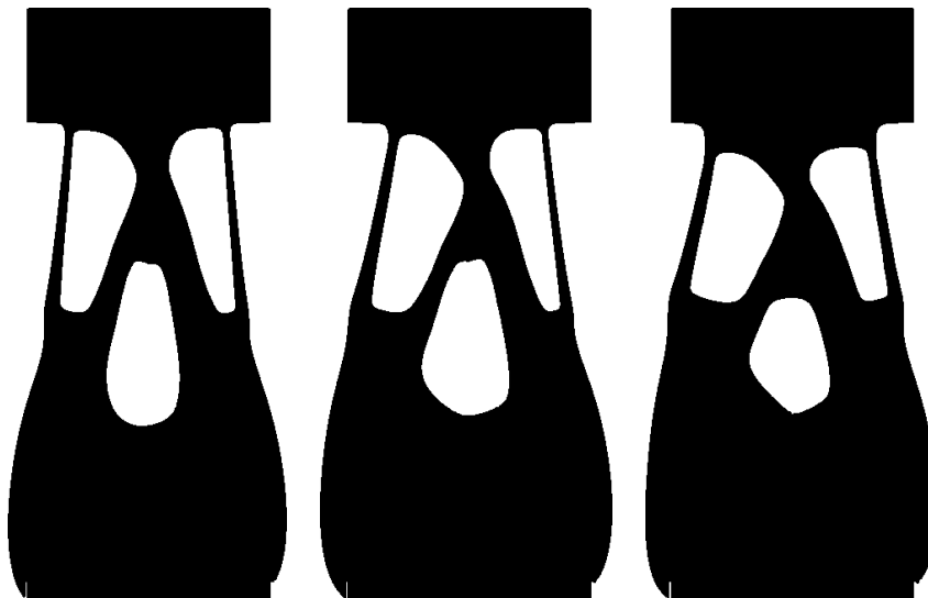
Fig. 5.19: Comparison of results using the set-up from Fig. 5.18. Left: Result from Algorithm 4.10 for the expectation based model. Middle: Result from Algorithm 4.10 for the expected excess model (3.42). Right: Result obtained for the expected excess model (3.40) with the barrier approach and Algorithm 4.11.
