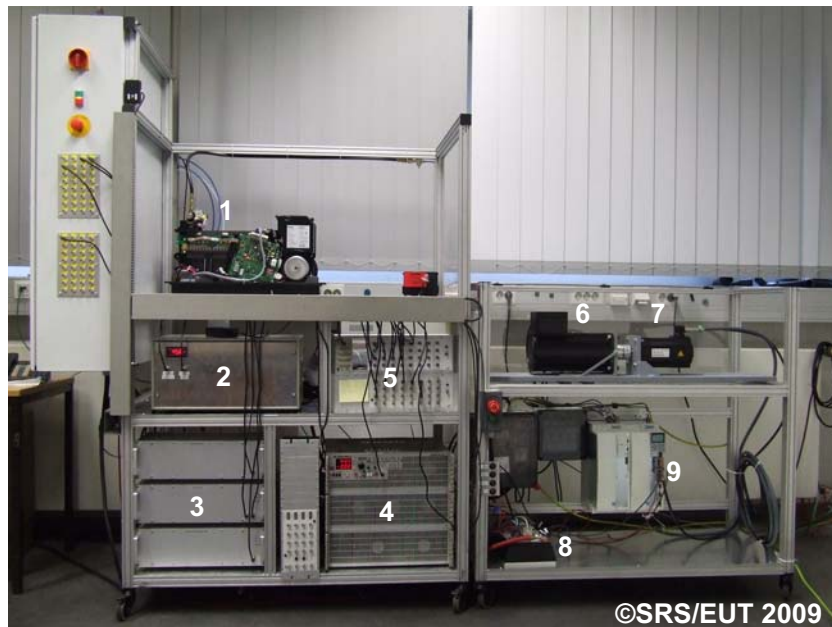
Figure 2.2: The Hardware-in-the-Loop test rig at the Chair of Dynamics and Control at the University of Duisburg-Essen. 1. Fuel cell system, 2. SuperCaps, 3. DC/DC-converters, 4. Power sink, 5. I/O-acquisition board, 6. Drive-motor, 7. Load-motor, 8. Drive-motor controller, 9. Load-motor controller
