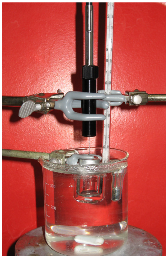
Fig. IV.3.1: Head-space sampling (HS) of urine for SPME-CG-MS (solid-phase microextraction gas chromatography and mass spectrometry) analysis, showing the sampling of dd H 2 O as a blank.
