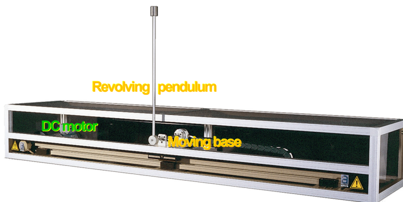
Figure 5.2: Inverted pendulum laboratory setup.
