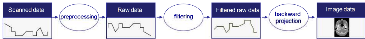
Figure 2-6: CT Internal reconstruction process (adapted from Prokop et al., 2006)
