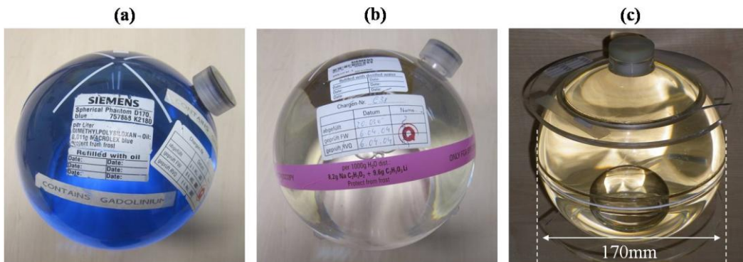
Figure 4.17: Spherical phantoms: (a) oil, (b) water, and (c) sugar dissolved in water
