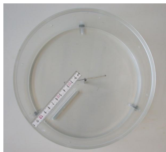
Fig. 2.3: Flight chamber for flight performance tests corresponding to the construction drawing without LED lighting; a = top view, b = lateral view.
