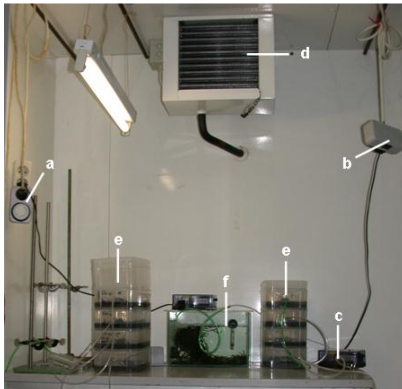
Fig. 2.1: Climate chamber equipped with species-specific breeding aquaria for Trichoptera; a = timer for lighting, b = power supply for diaphragm pump, c = diaphragm pump, d = cooling unit, e = aquaria towers, and f = food aquarium.
